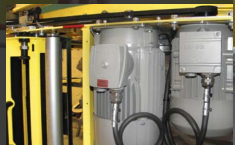
EPS: Electronic Pre-stretch System
