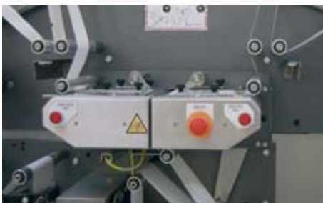
Automatic splice unit using adhesive tape
