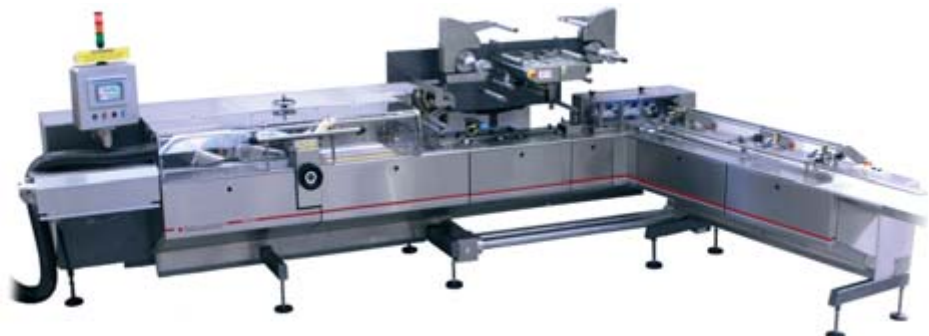
FT120 flow wrapper with AF including overhead transfer
