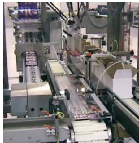
Dual loading of product into either multi-pack flow wrapper infeed or directly into a carton
