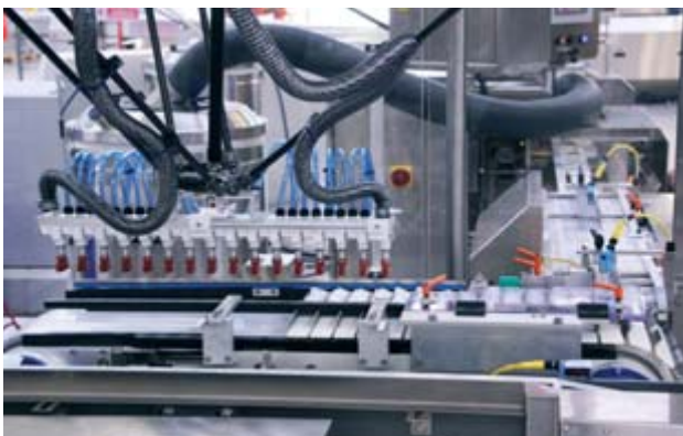
DRT collator and robotic 'multi-pack' loading
