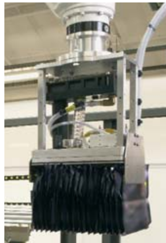
Mechanical / vacuum EOAT lifting a product on edge collation for shelf ready display
